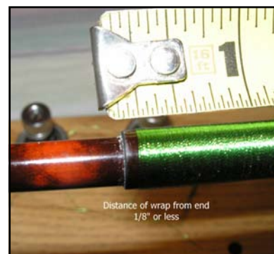
Photo #4: Distance of wrap from end
