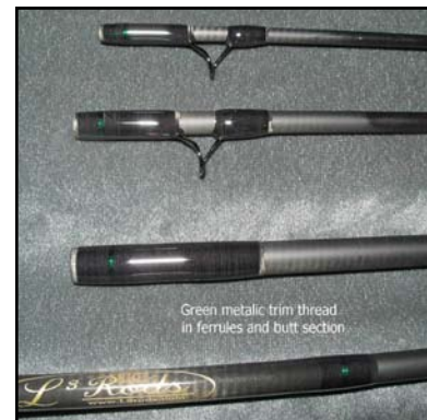
Green metallic trim thread in ferrules and butt section.
