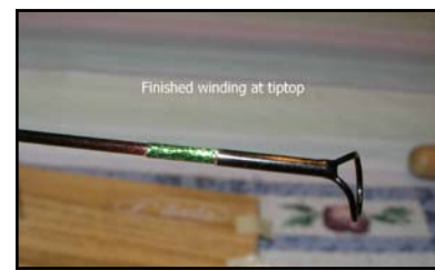
Finished winding of tiptop.
