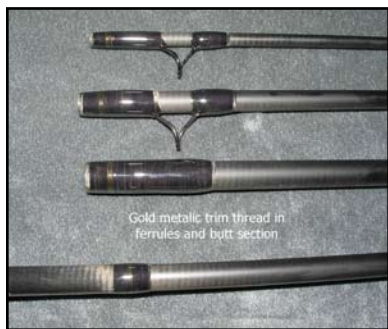
Gold metallic trim thread in ferrules and butt section.
