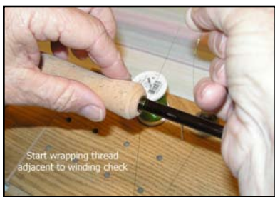
Photo #1: Start wrapping thread adjacent to winding check
