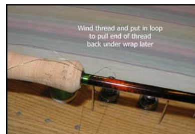
Photo #3: Wind thread and put in loop.
