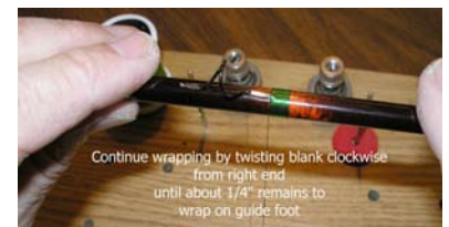
Photo 6: Continue wrapping by twisting blank clockwise from right end until about \frac{1}{4} " remains to wrap on guide foot.
