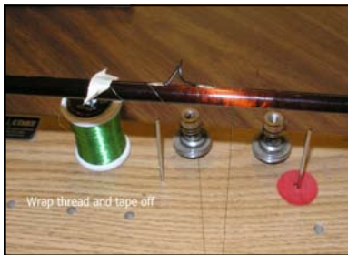
Photo 1: Wrap thread and tape off
