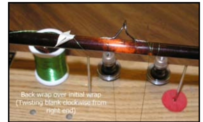
Photo 2: Back wrap over initial wrap (Twisting blank clockwise from right end)
