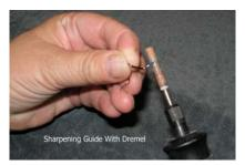
When sharpening the guides with the Dremel tool and the needle file, sharpen both the top and the bottom of each guide foot. Make sure that you do not leave any metal burrs on top of the foot (which would cut the thread) or on the bottom of the foot (which would dig into the blank and cause the blank to break in that location). Be cautious not to sharpen too quickly when using the Dremel tool because the metal in the guide may burn and the tip of the guide will be destroyed.
