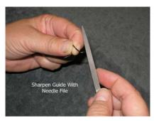
When the sharpening is complete, the end of the guide will be quite sharp and the thread can transition onto the foot when wrapping without any gaps. When sharpening really small guides or the hook-keeper guide, you may need a pair of needle nose pliers to hold the guide. Taking the time to sharpening the guides properly will greatly simplify the guide application.
