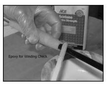
reside (see photo: "epoxy for winding check"). Next, slide the winding check down the blank onto the fresh epoxy until it rests next to the cork
