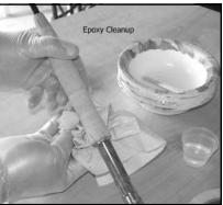
(see photo: Epoxy Cleanup). Prior to epoxy cleanup with acetone, make sure to align the center line of the slot of the reel seat with the spine (or spline) mark that you made earlier above the handle.
