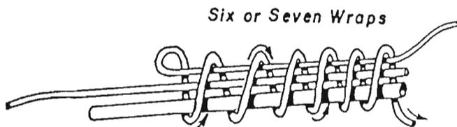
2. Hold the fly line, tube, and tag end of the leader together in your left hand. Now start wrapping the tag end of the leader around the fly line, tube, and standing part of the leader, working from left to right (toward the tag end of the fly line). The first turn must cross over the leader and start back toward the end of the fly line. For purposes of illustration, we have separated each wrap, but they should be made close together in tightly packed concentric circles.
